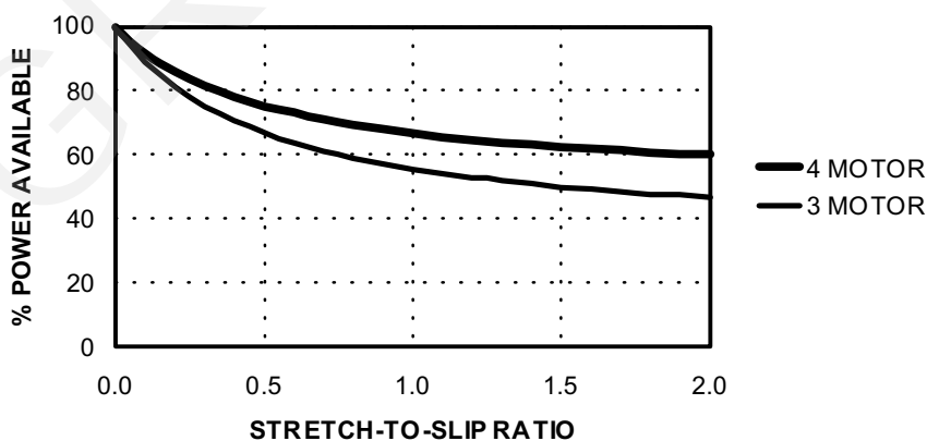
Fig. 4. Power available before overload occurs as a function of stretch and slip.
